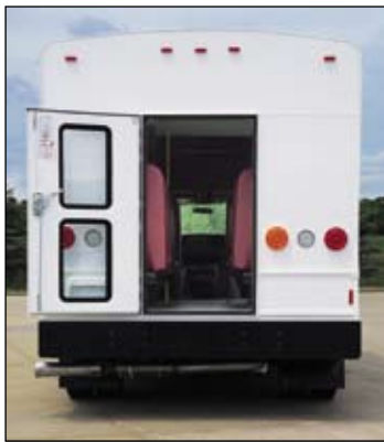
Rear emergency door and FMVSS exterior lights
